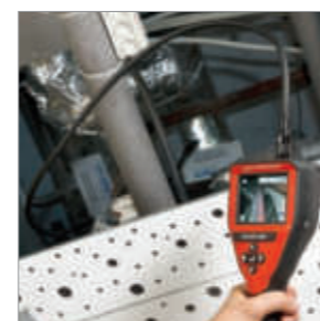
Camera head with high-performance LEDs
