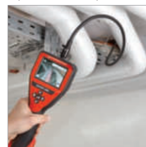
Inspection of hollow spaces
